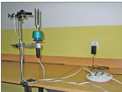
Fig. 4. Setup for registering sound amplitude as a function of angle of fork rotation.
