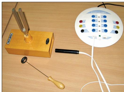
**Fig. 2. Tuning fork on a resonance box, sound detector, and a measuring console CoachLab II.<sup>3</sup>**
